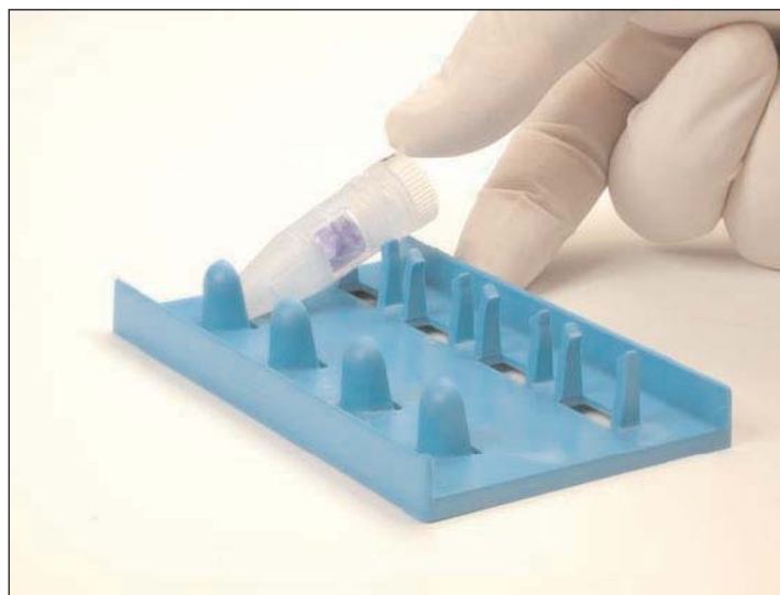
Figure 1: Insertion of the IBI FlexTube in the provided supporting tray. The arrow on the cap should be pointing upwards.
